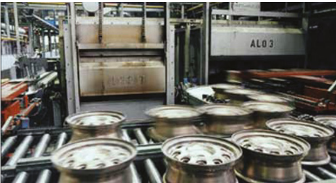
Aluminium industry: curing oven for wheel rims
